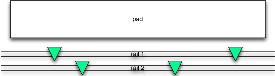
Reclaimers run on rails beside the pads. There can be multiple parallel rails, and multiple reclaimers on each rail. Reclaimers on the same rail can not pass each other, they have to stay in the same order. Reclaimers on separate rails are free to move past each other.
