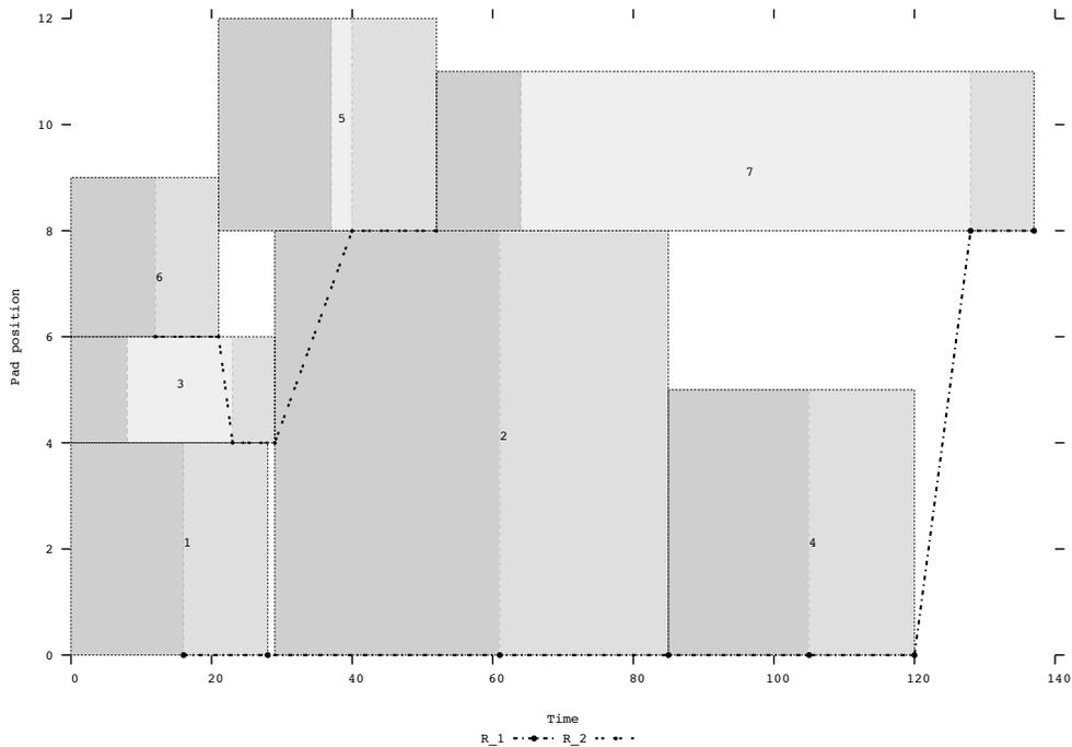
Figure 1: Pad diagram showing stacking, dwell, and reclaiming for each stockpile, as well as the path of the reclaimers.
